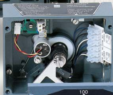
add feedback module at any time (switches and/or 4/20 transmitter)
